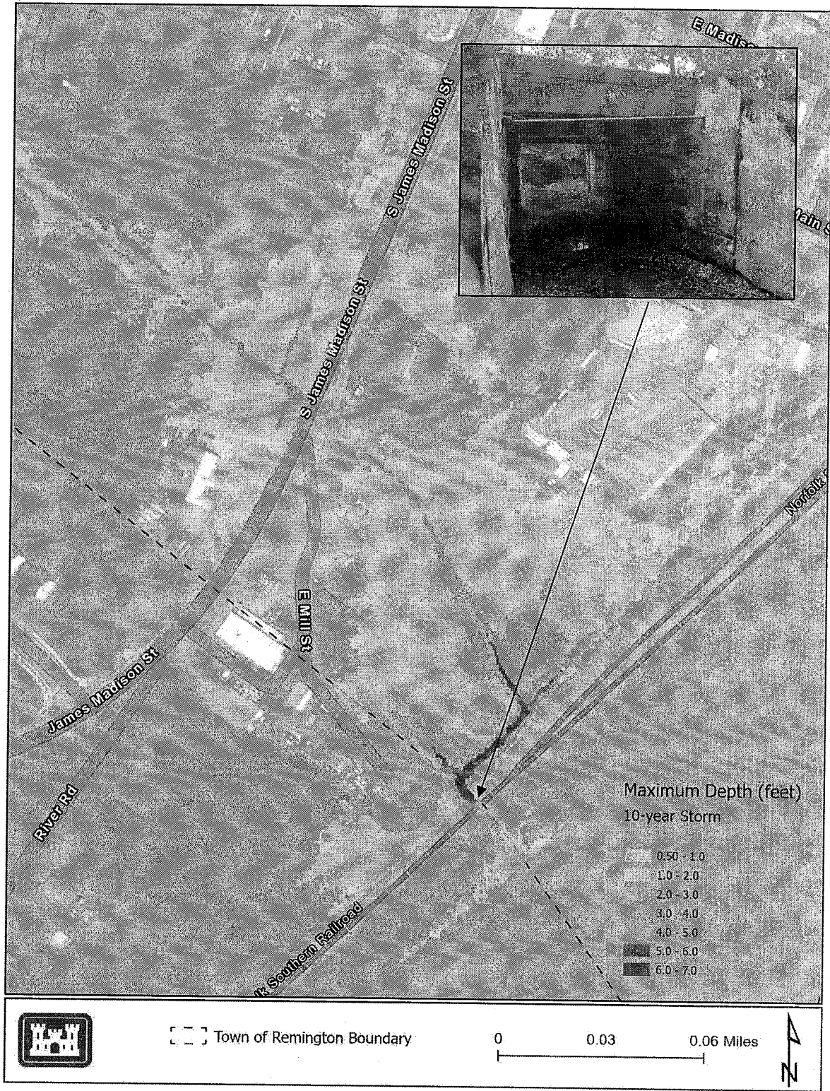
FIGURE 4.8: 10-YEAR FLOODING IN FOCUS AREA 4
